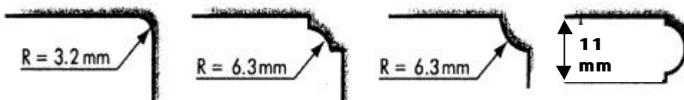
Blade N°1 Blade N°5 Blade N°8 Blade N°11 Different measures exist for various radius and width.
